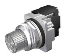
30mm Command/52, Chrome Finish Heavy Duty, Watertight/Oiltight Complete Metal Unit Illuminated Indicator Light Transformer type, 600V AC LED Lamp, BA9s Glass Lens, Clear UL Listed, CSA Certified NEMA 1,3,3R,4,4X,12,13 & Automotive Standards
