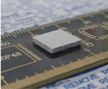
Tflex™ HD7.5 gap filler is a very soft silicone material in our high deflection series. With a thermal conductivity of 7.5W/ mk, Tflex™ HD7.5 is designed to provide superior pressure versus deflection characteristics. The material will provide minimal stress on components during application while maintaining low thermal resistance. As a result, less mechanical and thermal stresses will be experienced within your device.
