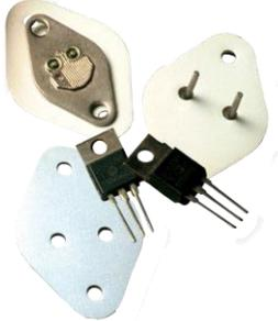
Tgard™ 500 is a medium thermal performance insulator pad consisting of a ceramic filled, high temperature, silicone rubber coated on electrical grade fiberglass. Tgard™ 500 has proven low thermal resistance after reliability and shows no delamination.
