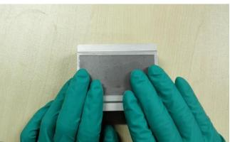
5. The thermal solution with Tgon<sup>TM</sup> 800A1 is now ready for final assembly.
