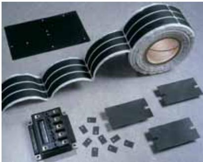
Bergquist Q-Pad 3 eliminates problems associated with thermal grease such as contamination of electronic assemblies and reflow solder baths. Q-Pad 3 may be installed prior to soldering and cleaning without worry. When clamped between two surfaces, the elastomer conforms to surface textures thereby creating an air-free interface between heat-generating components and heat sinks.
