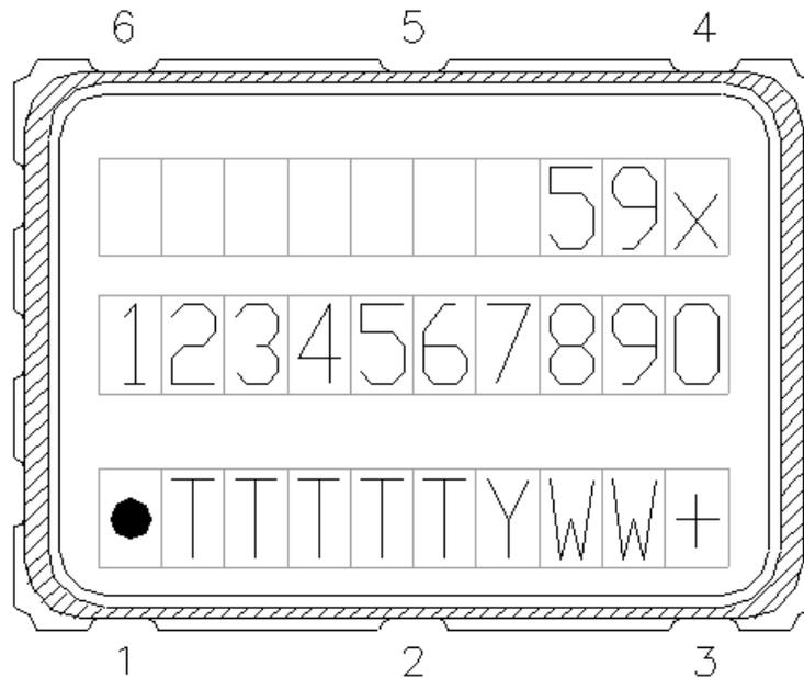
**Figure 6. Top Mark Specification**
