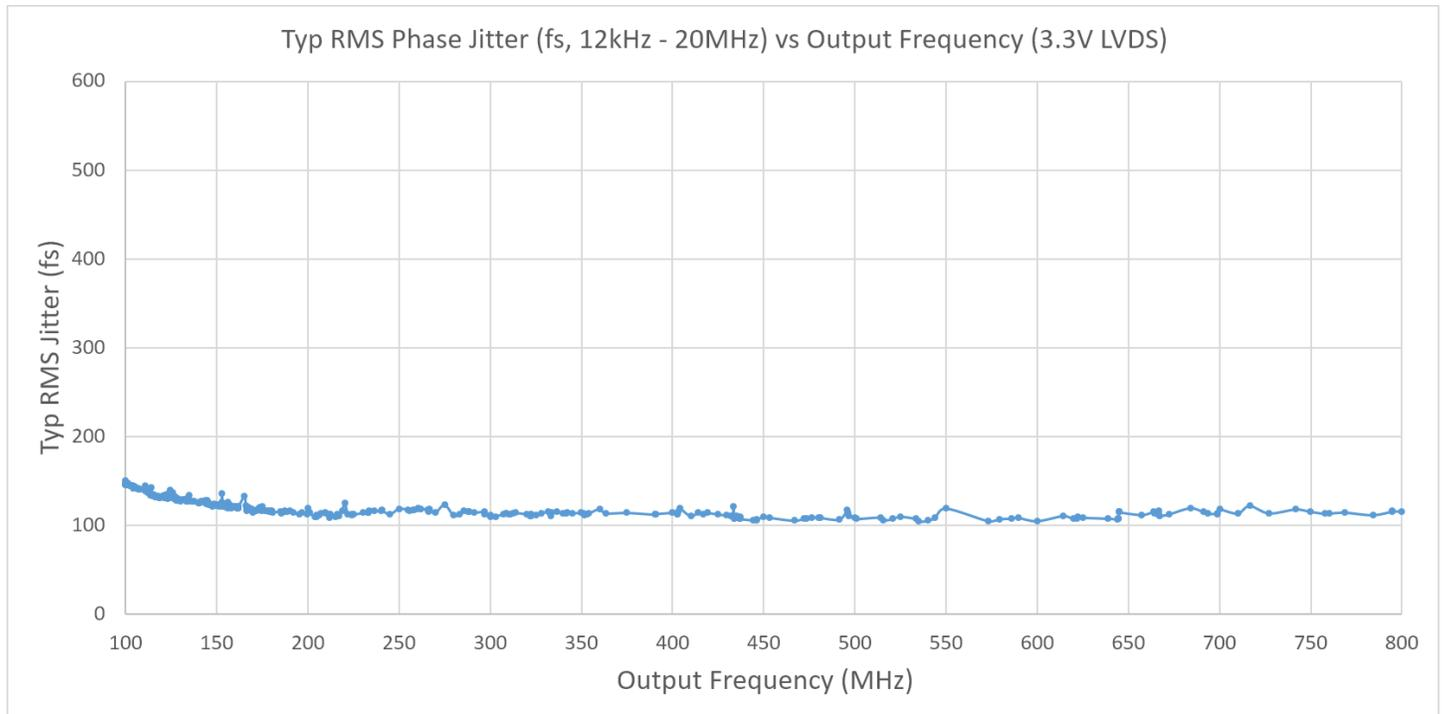
Phase jitter measured with Agilent E5052 using a differential-to-single ended converter (balun or buffer). Measurements collected for >700 commonly used frequencies. Phase noise plots for specific frequencies are available using our online [Oscillator Phase Noise Lookup Tool](#).
