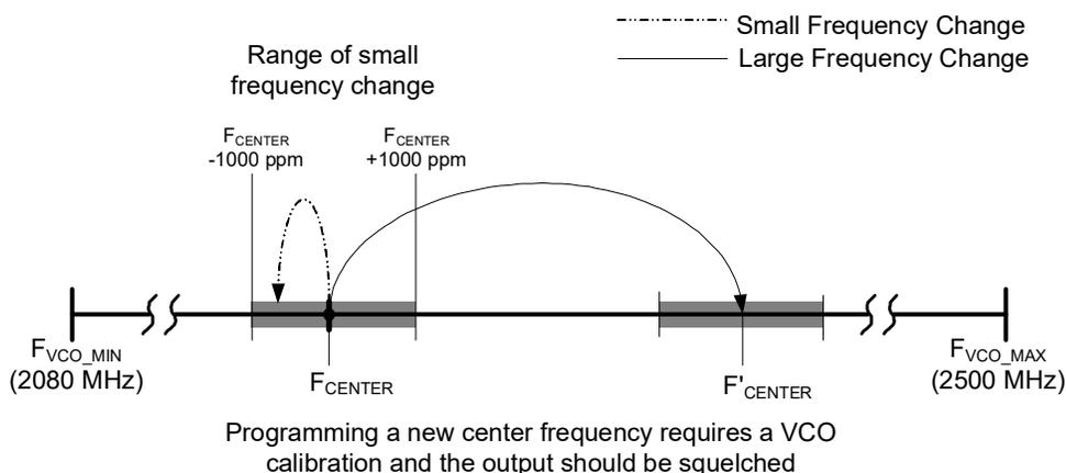
**Figure 2. Small vs. Large Frequency Change Illustration**
