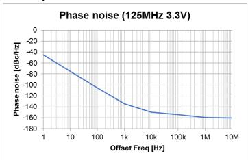
• Phase jitter: Typ. 90 fs (Frequency Offset: 12 kHz to 20 MHz) @125 MHz, 3.3 V
