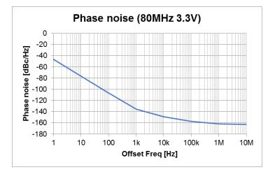
• Phase jitter : Typ. 100 fs (Frequency Offset: 12 kHz to 20 MHz) @80 MHz, 3.3 V
