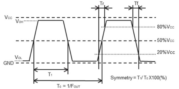
Fig.2 Clock Timing Chart (C-MOS Output)
