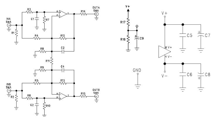
Figure 1: Complete Evaluation Board Schematic
