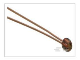
NTC Sensor Type: NTC Thermistor Lead Wire Length: 65 mm [2.559 in]Resistance (at 25°C):  $10 \text{ k}\Omega$ Resistance Tolerance (at 25°C):  $\pm 1\%$ Tolerance  $\beta$ -Value: 2%
