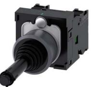
Coordinate switch, 22 mm, round, plastic with metal front ring, black, 2 switch positions, vertical latching, with mechanical interlocking, in O position, with holder, 1 NO, 1 NO, screw terminal, with laser labeling, upper case
