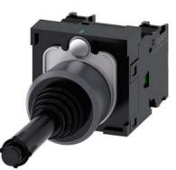
Coordinate switch, 22 mm, round, plastic with metal front ring, black, 2 switch positions, horizontal latching, with mechanical interlocking, in O position, with holder, 1 NO, 1 NO, screw terminal, with laser labeling, lower case
