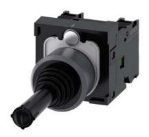
Coordinate switch, 22 mm, round, plastic with metal front ring, black, 2 switch positions, horizontal, momentary contact type, without mechanical interlocking in O position, with holder, 1 NO, 1 NO, screw terminal, with laser labeling, upper case and lower case, always upper case at the beginning of the word
