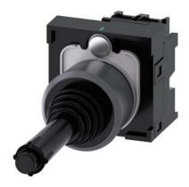
Coordinate switch, 22 mm, round, plastic with metal front ring, black, 2 switch positions, vertical latching, with mechanical interlocking, in O position, with holder, 1 NO, 1 NO, screw terminal,
