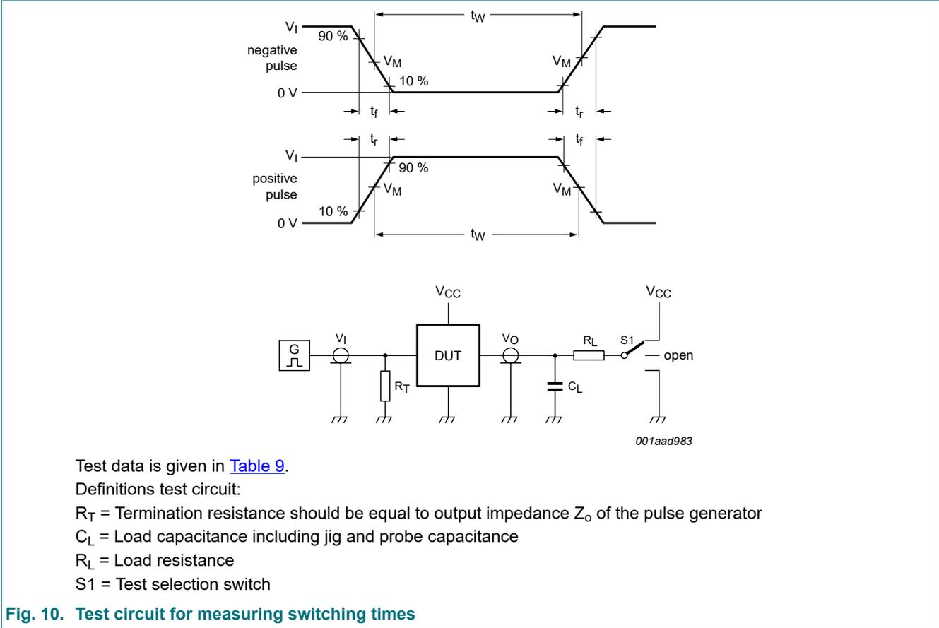
Fig. 10. Test circuit for measuring switching times
