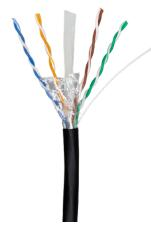
1 and 5 Gigabit (5GBASE-T) speeds up to 328 feet. Bandwidth tested up to 550 MHz. Supports PoE/PoE+/PoE++ (IEEE 802.3af/at/bt) 4PPoE up to 90W. Solid Copper Conductors ANSI/TIA 568 2.D, RoHS-3 compliant and cETLus certified. Bare copper is superior conductor material for data transmission and PoE use.
