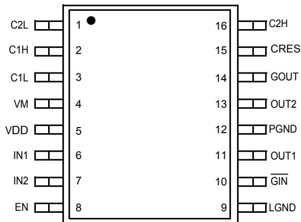
Figure 3. VMFP Pin Connections
