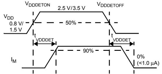
Figure 6. Low-Voltage Detection
