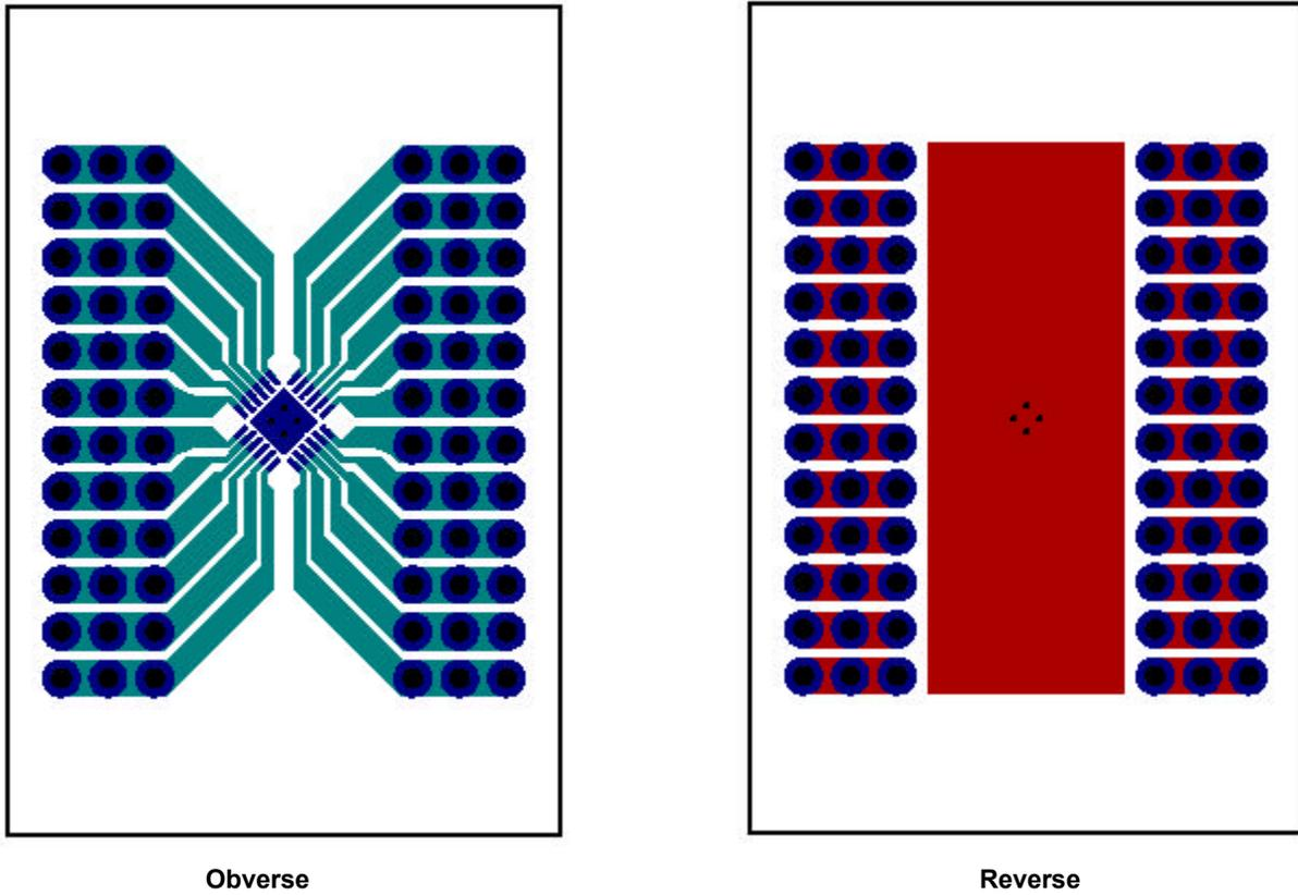
Figure 9. Recommended Heat Patterns for QFN24 EP
