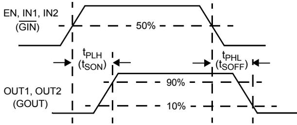
Figure 5.  $t_{PLH}$ ,  $t_{PHL}$ , and  $t_{PZH}$  Timing
