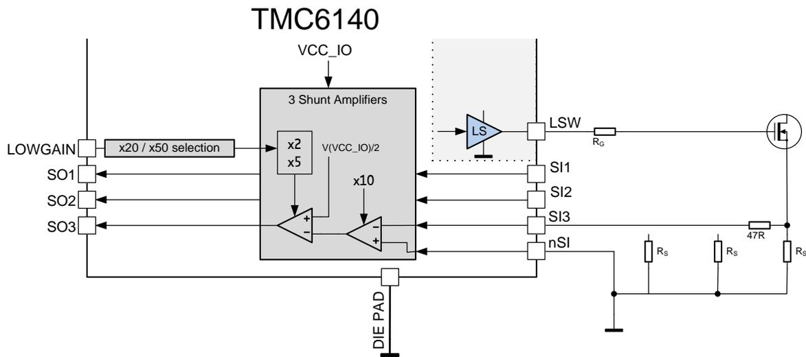
Figure 12: Shunt Amplifier setup for phase W
