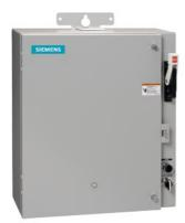
Pump control panel, Size 6, Three phase full voltage, Solid-state overload relay, OLR amp range 160-630A, 220-240V 50-60Hz/DC coil, Standard type contactor, 600A fusible disconnect, 600A/600V fuse clip, HOA Sel Sw. <(>&<)> Start P.B., Enclosure NEMA type 3/3R, Weather proof outdoor use
