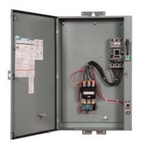
Pump control panel, Size 4, Three phase full voltage, Solid-state overload relay, OLR amp range 50-200A, 110-120/220-240VAC 60Hz coil, Standard type contactor, 150A circuit breaker, HOA Sel Sw. <(>&<)> Start P.B., Enclosure NEMA type 3/3R, Weather proof outdoor use
