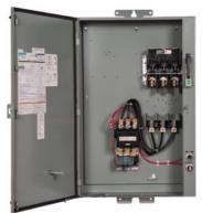
Pump control panel, Size 4, Three phase full voltage, Solid-state overload relay, OLR amp range 50-200A, 110-120/220-240VAC 60Hz coil, Standard type contactor, 200A fusible disconnect, 200A/250V fuse clip, HOA Sel Sw. <(>&<)> Start P.B., Enclosure NEMA type 3/3R, Weather proof outdoor use
