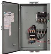
Pump control panel, Size 4, Three phase full voltage, Solid-state overload relay, OLR amp range 50-200A, 240V 50Hz / 277V 60Hz coil, Standard type contactor, 200A fusible disconnect, 200A/600V fuse clip, HOA Sel Sw. <(>&<)> Start P.B., Enclosure NEMA type 3/3R, Weather proof outdoor use
