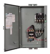
Pump control panel, Size 4, Three phase full voltage, Solid-state overload relay, OLR amp range 50-200A, 208VAC 60Hz coil, Standard type contactor, 200A fusible disconnect, 200A/600V fuse clip, HOA Sel Sw. <( $\times$ 8)> Start P.B., Enclosure NEMA type 3/3R, Weather proof outdoor use
