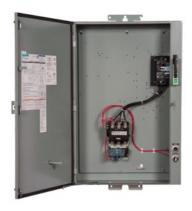
Pump control panel, Size 3 1/2, Three phase full voltage, Solid-state overload relay, OLR amp range 50-200A, 380-440/440-480V 50/60Hz coil, Standard type contactor, 125A circuit breaker, HOA Sel Sw. <(>&<)> Start P.B., Enclosure NEMA type 3/3R, Weather proof outdoor use
