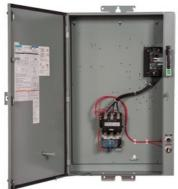
Pump control panel, Size 3 1/2, Three phase full voltage, Solid-state overload relay, OLR amp range 50-200A, 208VAC 60Hz coil, Standard type contactor, 125A circuit breaker, HOA Sel Sw. <(>&<)> Start P.B., Enclosure NEMA type 3/3R, Weather proof outdoor use
