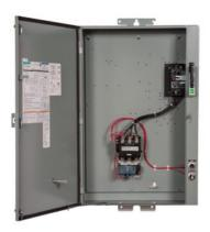
Pump control panel, Size 3, Three phase full voltage, Solid-state overload relay, OLR amp range 25-100A, 24VAC 50-60Hz coil, Standard type contactor, 100A circuit breaker, HOA Sel Sw. <(>&<)> Start P.B., Enclosure NEMA type 3/3R, Weather proof outdoor use
