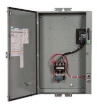
Pump control panel, Size 3, Three phase full voltage, Solid-state overload relay, OLR amp range 25-100A, 380-440/440-480V 50/60Hz coil, Standard type contactor, 100A circuit breaker, HOA Sel Sw. <(>&<)> Start P.B., Enclosure NEMA type 3/3R, Weather proof outdoor use
