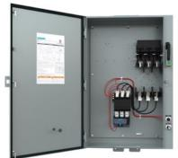
Pump control panel, Size 3, Three phase full voltage, Solid-state overload relay, OLR amp range 25-100A, 190-220/220-240V 50/60Hz coil, Standard type contactor, 100A fusible disconnect, 100A/600V fuse clip, HOA Sel Sw. <(>&<)> Start P.B., Enclosure NEMA type 3/3R, Weather proof outdoor use
