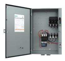
Pump control panel, Size 3, Three phase full voltage, Solid-state overload relay, OLR amp range 25-100A, 110V 50Hz / 120V 60Hz coil, Standard type contactor, 100A fusible disconnect, 100A/600V fuse clip, HOA Sel Sw. <(>&<)> Start P.B., Enclosure NEMA type 3/3R, Weather proof outdoor use
