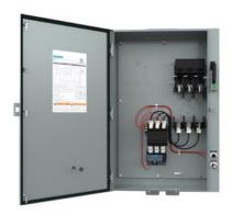
Pump control panel, Size 3, Three phase full voltage, Solid-state overload relay, OLR amp range 25-100A, 220-240/440-480VAC 60Hz coil, Standard type contactor, 100A fusible disconnect, 100A/600V fuse clip, HOA Sel Sw. <(>&<)> Start P.B., Enclosure NEMA type 3/3R, Weather proof outdoor use
