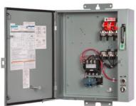
Pump control panel, Size 2 1/2, Three phase full voltage, Solid-state overload relay, OLR amp range 25-100A, 190-220/220-240V 50/60Hz coil, Standard type contactor, 60A fusible disconnect, 60A/250V fuse clip, HOA Sel Sw. <(>&<)> Start P.B., Enclosure NEMA type 3/3R, Weather proof outdoor use
