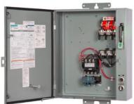
Pump control panel, Size 2, Three phase full voltage, Solid-state overload relay, OLR amp range 13-52A, 110V 50Hz / 120V 60Hz coil, Standard type contactor, 60A fusible disconnect, 60A/250V fuse clip, HOA Sel Sw. <(>&<)> Start P.B., Enclosure NEMA type 3/3R, Weather proof outdoor use
