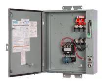
Pump control panel, Size 2, Three phase full voltage, Solid-state overload relay, OLR amp range 13-52A, 190-220/220-240V 50/60Hz coil, Standard type contactor, 60A fusible disconnect, 60A/600V fuse clip, HOA Sel Sw. <(>&<)> Start P.B., Enclosure NEMA type 3/3R, Weather proof outdoor use
