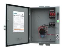
Pump control panel, Size 1 3/4, Three phase full voltage, Solid-state overload relay, OLR amp range 10-40A, 380-440/440-480V 50/60Hz coil, Standard type contactor, 60A fusible disconnect, 60A/600V fuse clip, HOA Sel Sw. <(>&<)> Start P.B., Enclosure NEMA type 3/3R, Weather proof outdoor use
