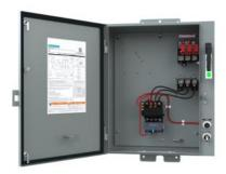
Pump control panel, Size 1, Three phase full voltage, Solid-state overload relay, OLR amp range 5.5-22A, 240V 50Hz / 277V 60Hz coil, Standard type contactor, 60A fusible disconnect, 60A/600V fuse clip, HOA Sel Sw. <(>&<)> Start P.B., Enclosure NEMA type 3/3R, Weather proof outdoor use
