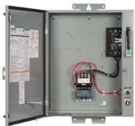
Pump control panel, Size 1, Three phase full voltage, Solid-state overload relay, OLR amp range 3-12A, 240V 50Hz / 277V 60Hz coil, Standard type contactor, 10A circuit breaker, HOA Sel Sw. <(>&<)> Start P.B., Enclosure NEMA type 3/3R, Weather proof outdoor use
