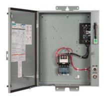
Pump control panel, Size 1, Three phase full voltage, Solid-state overload relay, OLR amp range 3-12A, 220-240/440-480VAC 60Hz coil, Standard type contactor, 10A circuit breaker, HOA Sel Sw. <(>&<)> Start P.B., Enclosure NEMA type 3/3R, Weather proof outdoor use
