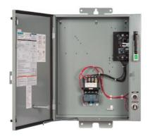
Pump control panel, Size 1, Three phase full voltage, Solid-state overload relay, OLR amp range 0.75-3.4A, 110V 50Hz / 120V 60Hz coil, Standard type contactor, 3A circuit breaker, HOA Sel Sw. <(>&<)> Start P.B., Enclosure NEMA type 3/3R, Weather proof outdoor use
