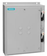
Duplex starter w/o alternator Size 4 Three phase full voltage Solid-state overload relay OLR amp range 50-200A 110VAC 50Hz / 120VAC 60Hz Coil Combination type Two 200A disconnect switches Encl NEMA type 4X 304 S. Steel Water/dust tight non-corrosive
