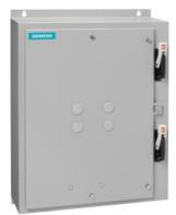
Duplex starter w/o alternator Size 4 Three phase full voltage Solid-state overload relay OLR amp range 50-200A 110VAC 50Hz / 120VAC 60Hz Coil Combination type Two 200A disconnect switches Enclosure NEMA type 1 Indoor general purpose use
