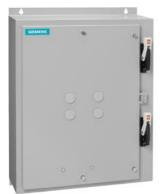
Duplex starter w/o alternator, Size 3 1/2, Three phase full voltage, Solid-state overload relay, OLR amp range 50-200A, 190-220/220-240V 50/60Hz coil, Combination type, Two 125A circuit breakers, Enc NEMA type 4 painted steel, Water/dust tight for outdoors
