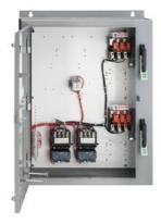
Duplex starter with alternator Size 3.5 Three phase full voltage Solid-state overload relay OLR amp range 50-200A 110VAC 50Hz / 120VAC 60Hz Coil Combination type Two 200A disconnect switches Enclosure NEMA type 4/12 Water/dust tight weather proof
