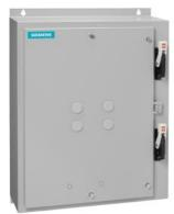
Duplex starter w/o alternator Size 3 Three phase full voltage Solid-state overload relay OLR amp range 25-100A Combination type Two 100A disconnect switches Encl NEMA type 4 painted steel Water/dust tight weather proof
