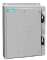
Duplex starter w/o alternator, Size 3, Three phase full voltage, Solid-state overload relay, OLR amp range 25-100A, 208VAC 60Hz coil, Combination type, Two 100A circuit breakers, Enclosure NEMA type 12, Dust/drip proof for indoors
