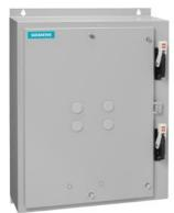
Duplex starter w/o alternator Size 3 Three phase full voltage Solid-state overload relay OLR amp range 25-100A 24VAC 50-60Hz Coil Combination type Two 100A disconnect switches Enclosure NEMA type 4/12 Water/dust tight weather proof
