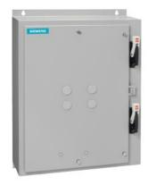
Duplex starter w/o alternator, Size 2, Three phase full voltage, Solid-state overload relay, OLR amp range 13-52A, 24VAC 50-60Hz coil, Combination type, Two 50A circuit breakers, Enclosure NEMA type 1, Indoor general purpose use
