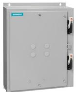
Duplex starter w/o alternator Size 2 Three phase full voltage Solid-state overload relay OLR amp range 13-52A 110VAC 50Hz / 120VAC 60Hz Coil Combination type Two 60A disconnect switches Enclosure NEMA type 1 Indoor general purpose use
